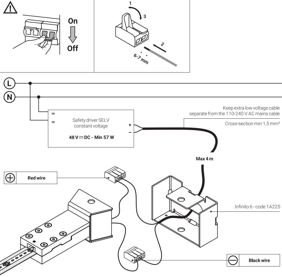
Infinito 12 - Example of connection with remote power supply kit
