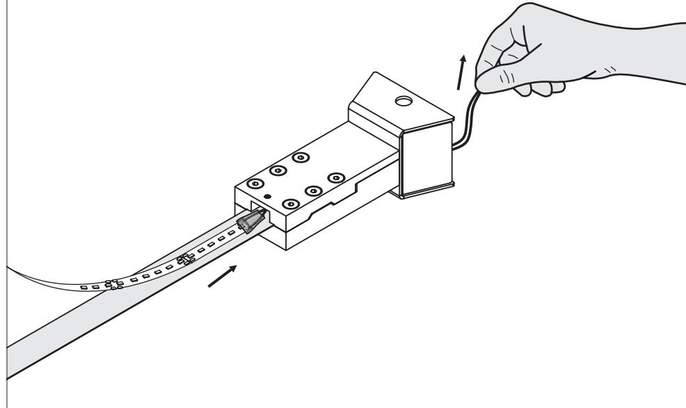
Infinito 6 - Example of connection with remote power supply kit
