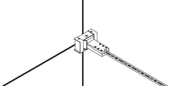
Infinito 6 - Infinito 12 - Example of connection with power kit with plug
