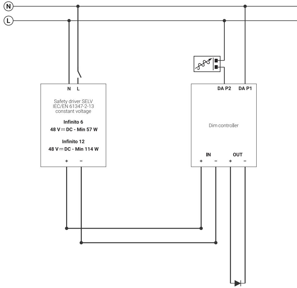
**Example connection (optional) for dimming 1-10V**
