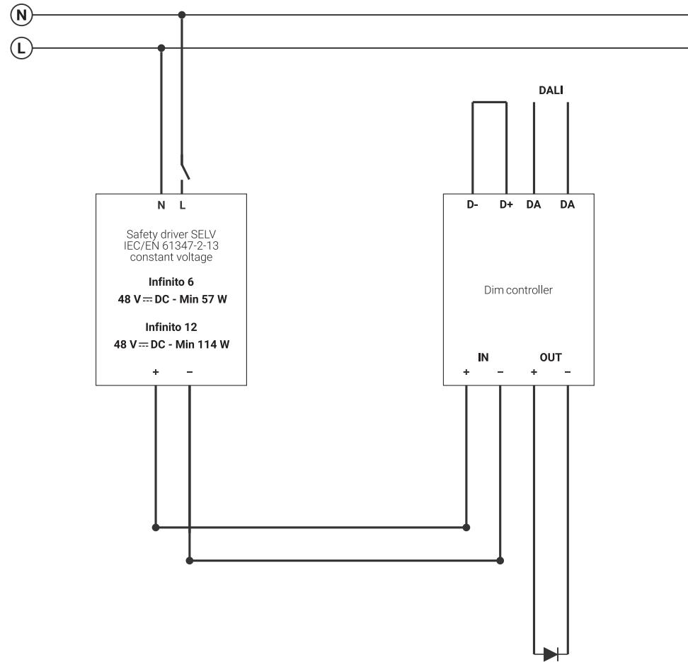
**Example connection (optional) for dimming TRIAC/IGBT**
